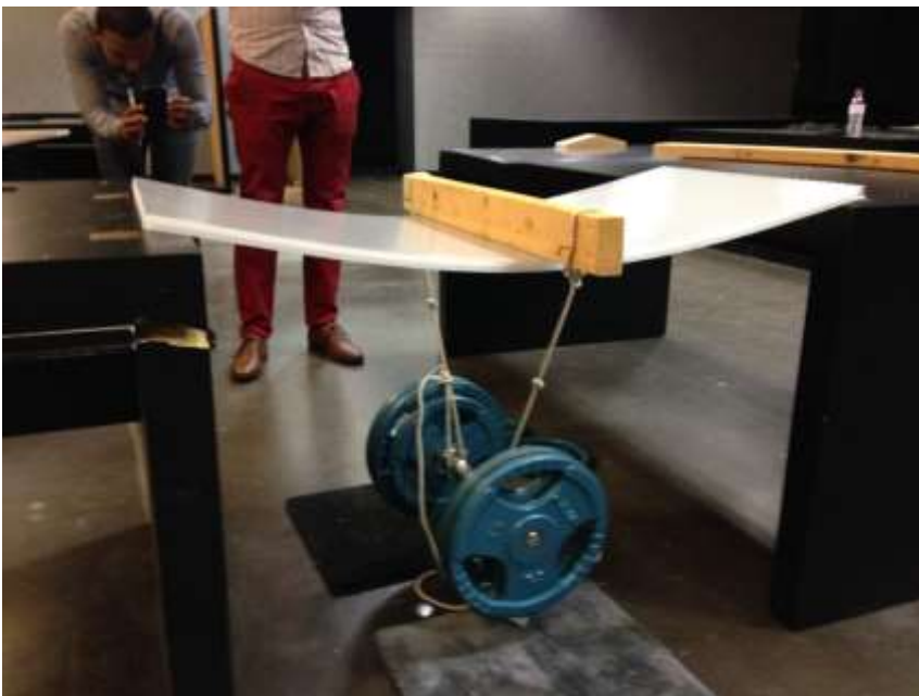
Figure 5 – Direct bending test of sheeting (strong axis test shown)
