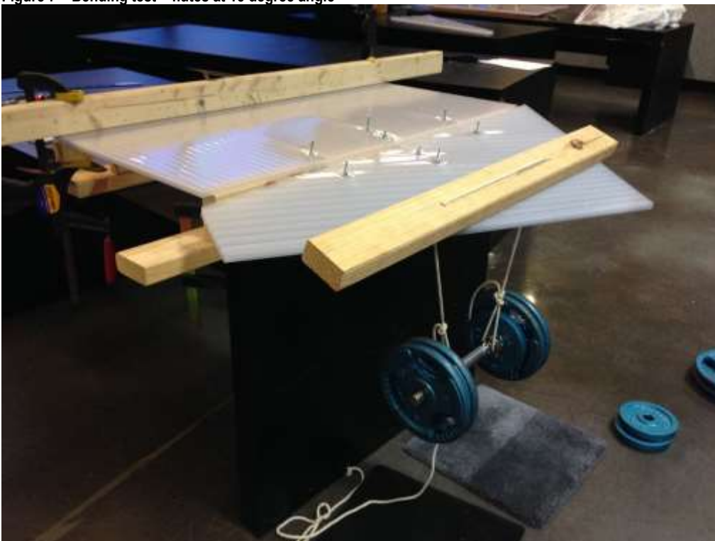
Figure 7 – Bending test – flutes at 15 degree angle
