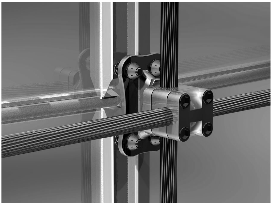
Figure 4. Cable Net – Unitized Frame Connection
