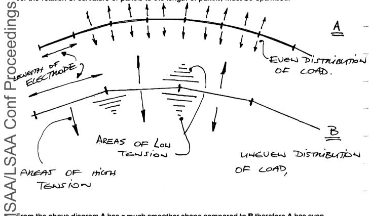
From the above diagram A has a much smoother shape compared to B therefore A has even loading throughout the seam where B has much higher loading at the centre of each weld. This can cause uneven tension and hence wrinkles will occur in this region of the structure.
