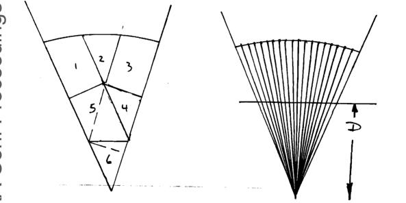
Also the more welds required, produce large ridges of "squeeze out" (a bi-product of the weld). This forms a ridge to both sides of the weld. This traps dirt and can give moulds a rough surface to grip to.Over welding an area such as "D" above can considerably weaken the strength of the fabric - i.e. - all P.V.C is pushed away from weld and hence only base fabric remains this fabric has no weldability.
