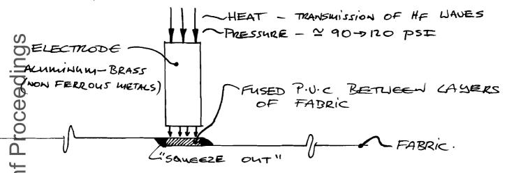
In order to truly test a welded seam (etc) a destructive test must be performed - "(A peel test)" when the weld is pulled apart the P.V.C shall be completely removed (100%) from either surface or in a combination from both surfaces, to expose the base fabric.
